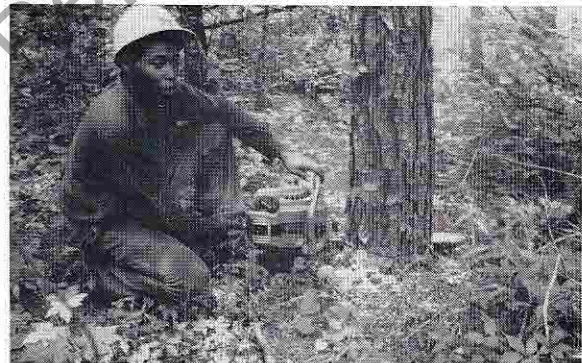
Here, a cutter uses an XL-800 with flush-cut handle to slice through a small tree close to the ground. The light weight insures less operator fatigue.
