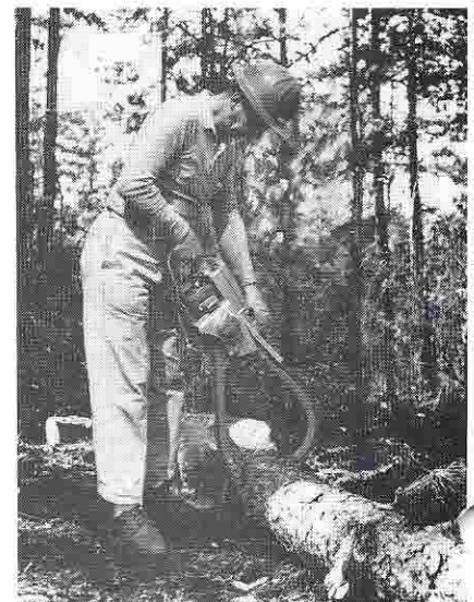
The new C-5GB chain saw comes equipped to use the new bow attachment.
