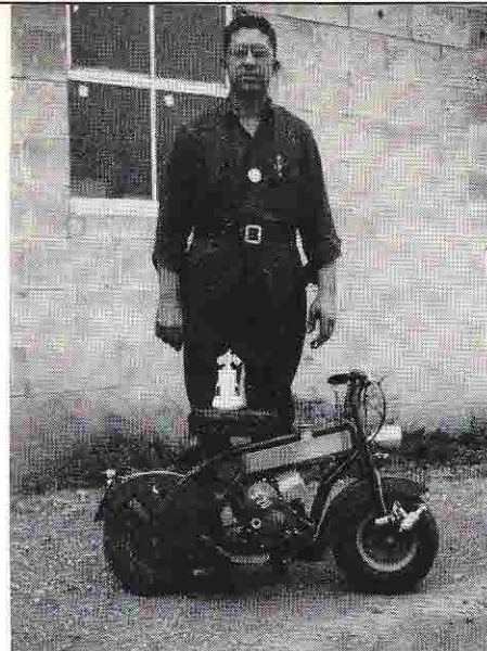
Anthony Arnold of Marietta, Ohio, and the scooter he built around a 5-20 chain saw engine.
