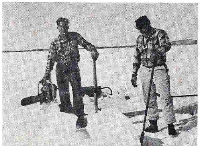
MAKING ICE DUST IN ALASKA, Neal Johnsen, left, and Roger Butler, cut huge cakes of crystal clear ice with their trusty model 17 Homelite. They pack it in sawdust to keep it frozen.
