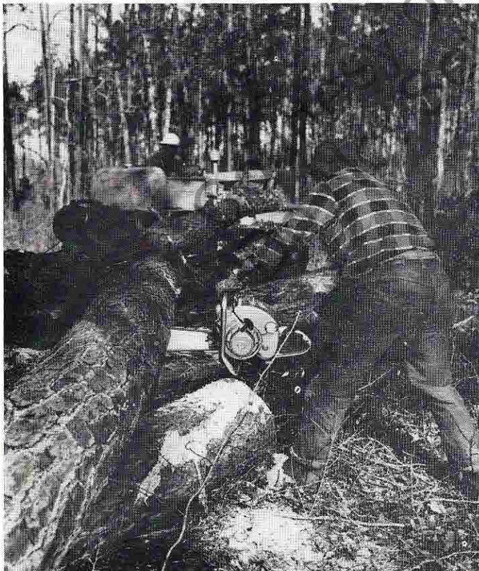
BELOW . . . The new WIZ, in the hands of an experienced operator, cuts through the logs easily and quickly. The new Homelite guide bar is induction-hardened and hard tipped to give long wear and to reduce "down time."
