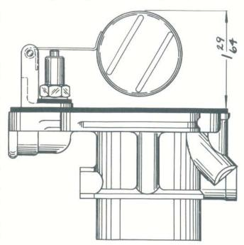
Needle and Seat, clean their seating surfaces with a soft clean cloth. Place Inlet Needle in its Seat and tap very lightly, turning Inlet Needle with thumb and forefinger several times to reseat. Reinstall, and if proper level is not maintained, install a new Inlet Needle, Seat and Gasket (A). DO NOT CHANGE GASOLINE LEVEL FROM MANUFACTURERS SPECIFICATIONS.
