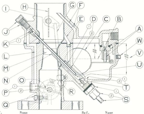
Ref. Name No. 4 Inlet Needle, Seat & Gasket B Fuel Level C Float
