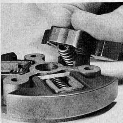
Fig. HL88—To install late type clutch shoe and spring, place spring between shoe and plate as shown, hook shoe onto plate and push shoe down into place.
