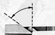
Fig. 7—Filing angles for chipper type chain in average use.
