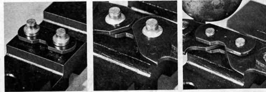
3. Put preset part on flat surface. 4. Install chain on new part. 5. Dimple on tie strap faces out. Form rivet head with hammer.
