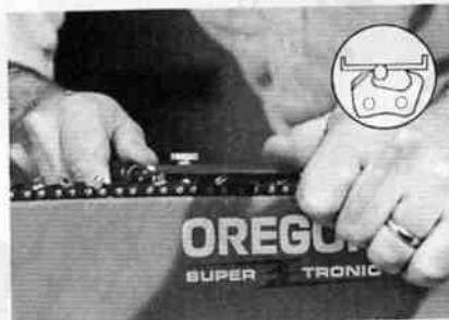
Fig. 11—Filing 80 chain top plates. Make sure chain is tensioned tight before filing.
