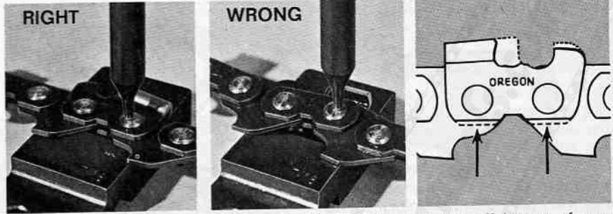
1. Fit chain into smallest slot of Chain Breaker so cutter is on top. Punch out rivets of damaged part. 2. File off bottom of new part to match worn parts. File new cutter back to match worn cutters.
