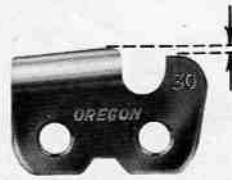
Check depth gauges every 3rd or 4th sharpening.
