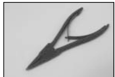
Snap ring pincer for external snap rings of starting system 946 101 010
