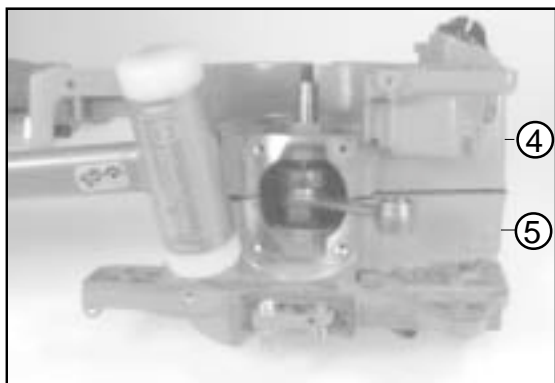
11-03 Removing the crankcase After removing the attachment screws, separate the crankcase using a plastic hammer.
