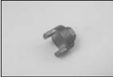
Mounting tool for clutch hub 944 500 680
