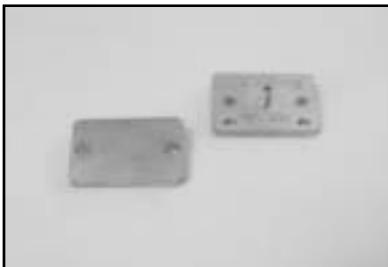
Sealing plate for leakage test of crankcase 944 603 020 / 944 603 030
