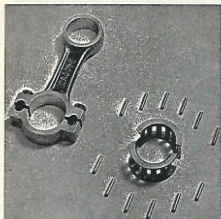
Fig. SK15—Connecting rod and crankpin bearing typical of those used in some models. Note matched notched corners on bearing cage flanges.
