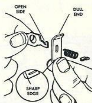
Fig. SK29-View showing assembly of friction shoe components.
