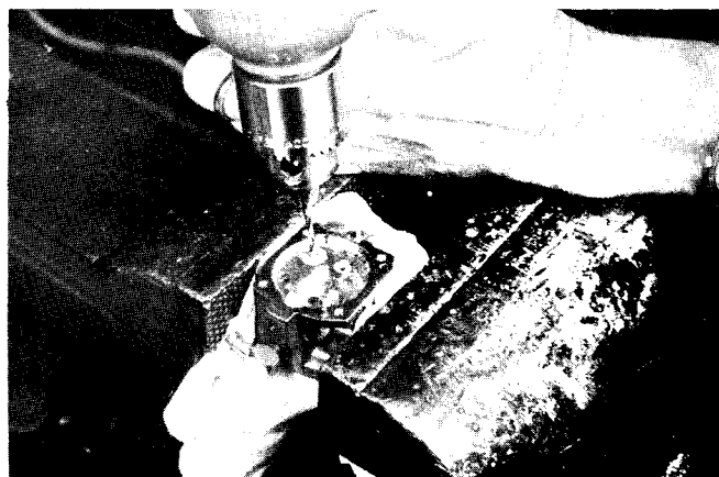
Fig. 63 — Drilling Welch Plugs Prior to Removal
