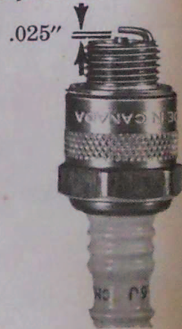
FIGURE 18 Spark Plug Gap
