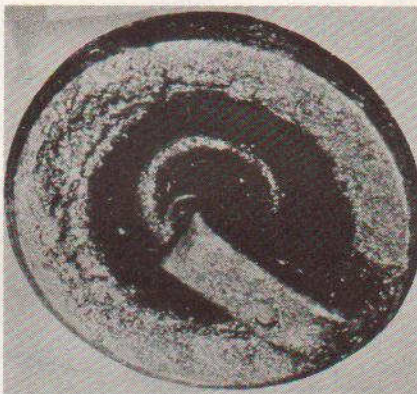
Fig. S4—Damp or wet black carbon coating over entire firing end of plug. Could be caused by rich carburetor mixture, too much oil in fuel, or low ignition voltage. Could also be caused by incorrect heat range (too cold) for operating conditions. Correct the defects or install a hotter plug.
