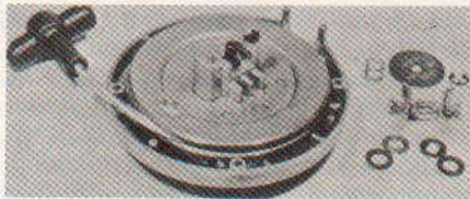
Fig. PR2-13—View of rewind starter with starter pawls and friction washers removed.
