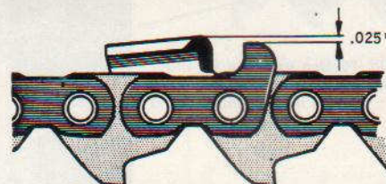
Fig. 14—Normal joint clearance is 0.025 inch as shown.
