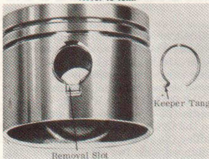
Fig. PR5-12—The tang on the piston pin keeper must be correctly installed in removal slot of the 2 inch diameter pistons.
