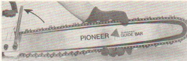
Fig. 5—Loosen the guide bar retaining nuts.
