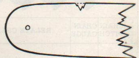
Fig. 28-Chipped rails can be caused by bar being pinched in cut or hitting bar with axe or wedge. Attempting to open the bar groove with screwdriver or similar object can also chip rail as shown.
