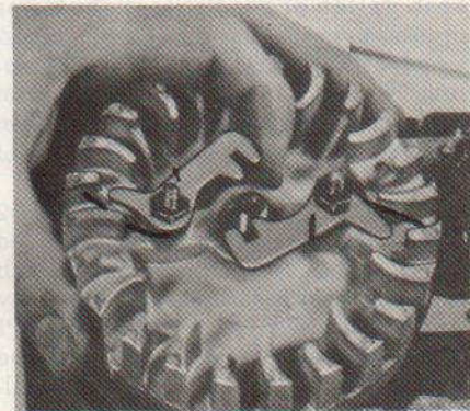
Fig. PR4-13—The starter pawls and springs should be installed as shown. A balance weight may be used with only one pawl assembly.
