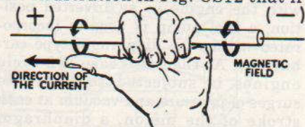
Fig. CS11—A field of magnetic force is always present around a wire through which current is flowing. The direction of magnetic force is related to the direction of electrical current as shown.
