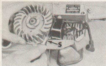
Fig. PR6-7—Armature air gap should be checked and adjusted using correct thickness of shim stock (S).
