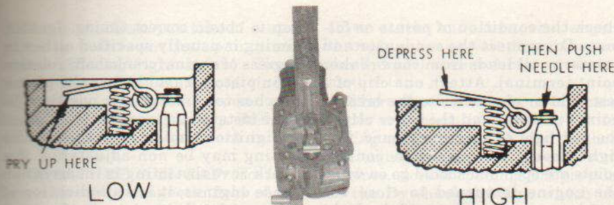
Fig. S12—Drawing showing proper adjustment of metering diaphragm lever.
