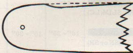
Fig. 25-Worn rails can be caused by chain tension too slack causing chain to crowd at this point. Under cutting with dull or damaged cutters or chain filled with insufficient joint can also cause this condition.
