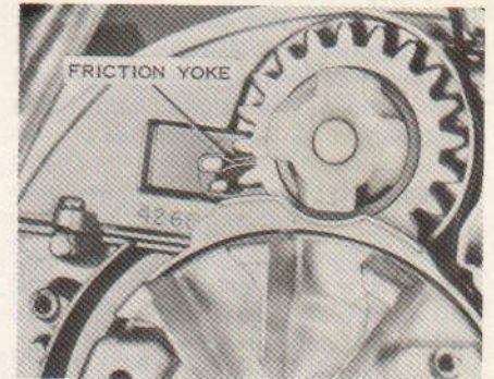
Fig. PR1-15—Friction yoke should be around upper projection as shown. Offset portion at outer end of yoke should be away from pinion.
