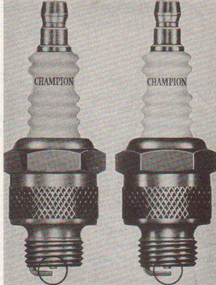
Fig. CS36—The two-cycle (left) differs from conventional plug in that the grounded electrode is shortened to minimize carbon fouling.
