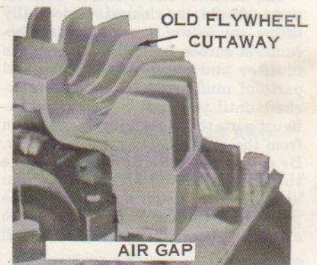
Fig. S19—Where armature core and ignition coil are located inside of flywheel, an old discarded flywheel can be cut away as shown to provide air gap adjustment fixture.
