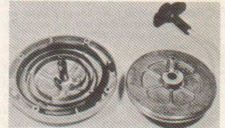
Fig. PR2-15—View of starter housing showing correct installation of rewind spring.
