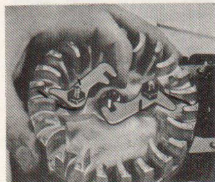
Fig. PR5-18—The starter pawls and springs should be installed as shown.
