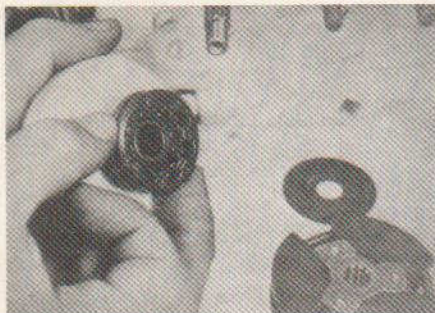
Fig. PR5-15A—The open side of floating sprocket should be away from clutch drum as shown.
