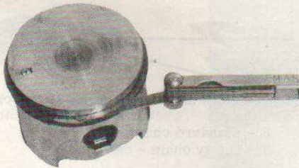
Fig. S30—Ring side clearance in groove should be measured with feeler gage as shown. Clearance should be within recommended limits and the same all the way around piston.
