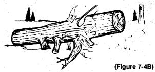
Log supported on one end: First cut from bottom (underbuck) 1/3 diameter of log to avoid splintering. Second, overbuck to meet first cut and avoid plnching. (Figure 7-4B)
