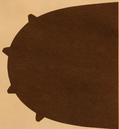
A-9 is \frac{3}{8} 9-tooth for MSA R-9 is \frac{3}{8} Lo Pro 9-tooth for MSR or SSR Radius 0.906"
