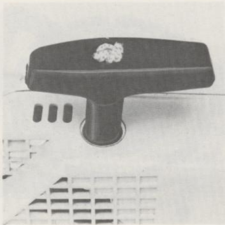
Starter grip firmly seated in rope bush
