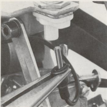
Pulling ground lead out of ignition stop switch
