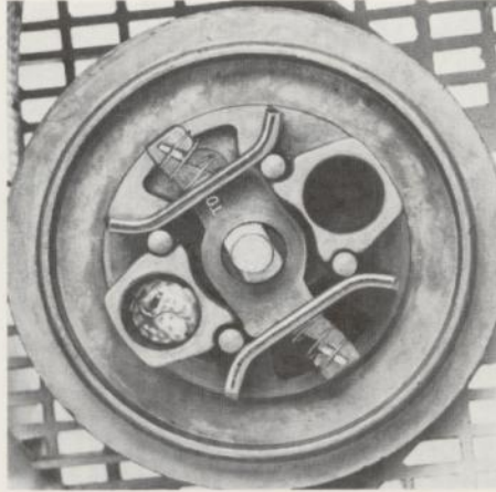
Friction shoe correctly positioned
