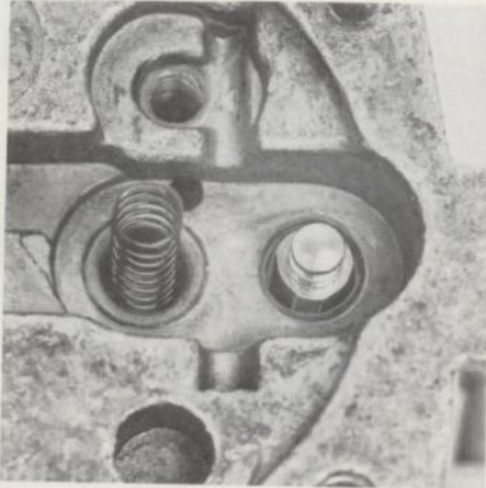
Inlet needle and helical spring in position
