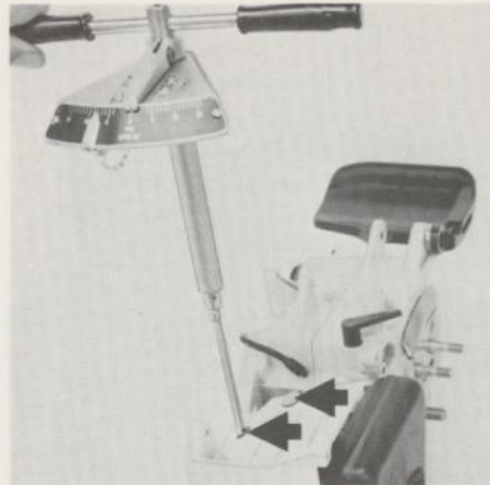
Tightening the muffler
