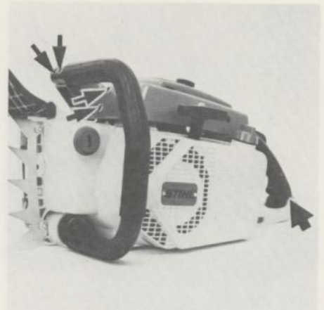
Bottom: Damper elements on handle frame
