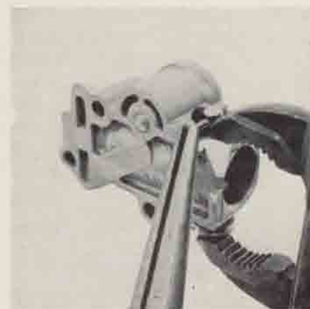
Depressing the regulating pin; removing the pin stop
