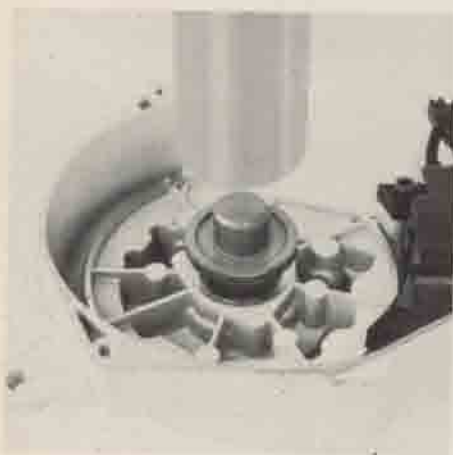
Forcing out the ignition end ball bearing:
