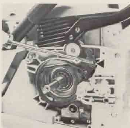
Middle and bottom: Unscrewing the hand guard
