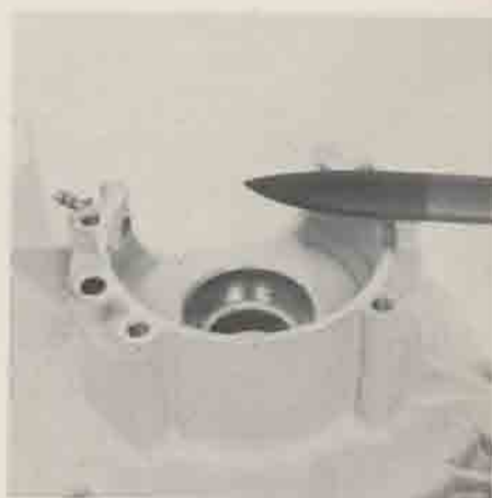
Bottom: Circlip installed
