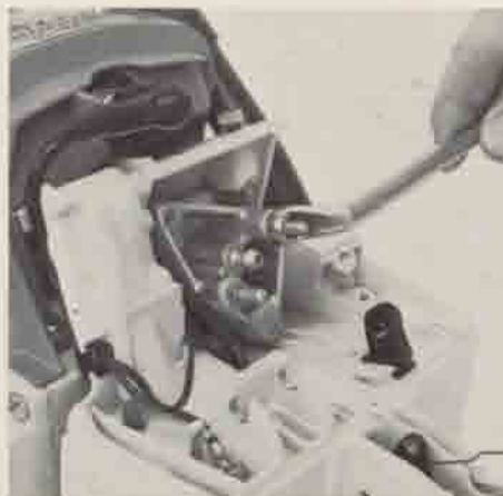
Bottom: Pressure-testing the carburetor
