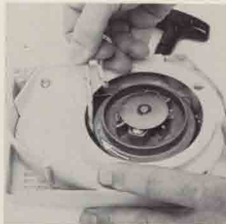
Tensioning the rewind spring
