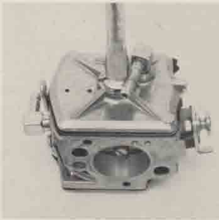
Loosening the pump-end cover
