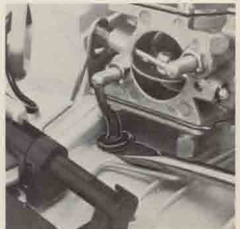
Prying out the hose
