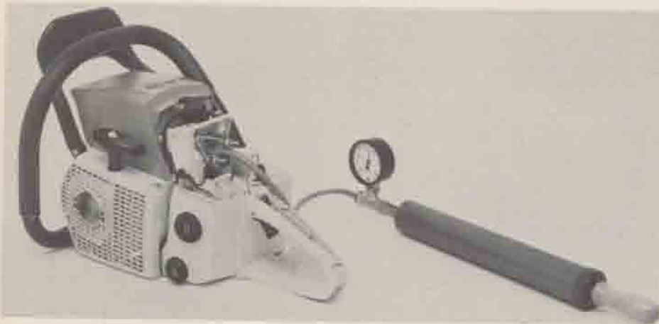
Leakage testing with vacuum pump
