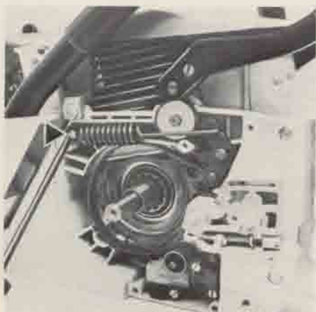
Unhooking the extension spring
