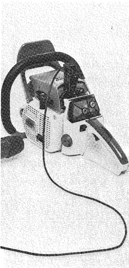
Flash directed at timing marks
