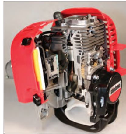
24.5cc Pushrod Overhead Valve Engine
