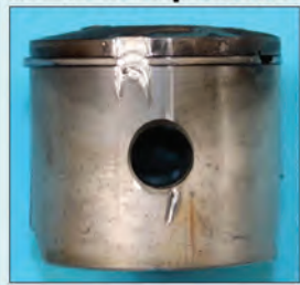
Wrist Pin Clip Came Out (Assembly Error)
