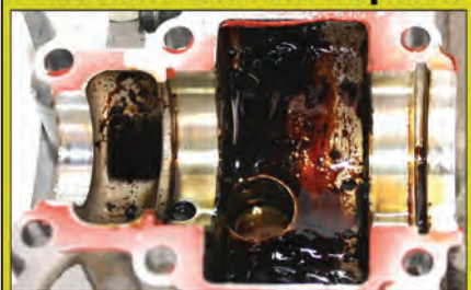
Key factor identifying stale fuel failures
