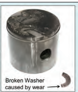
Wrist Pin Clip Came Out (Assembly Error)
