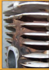
Blocked Cylinder Fins
