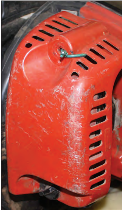
Wired on air filter cover
