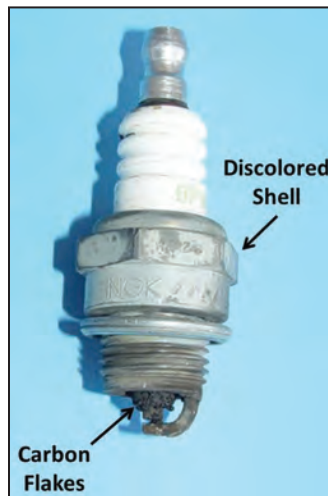
Overheated Spark Plug
