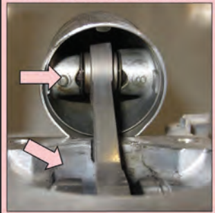
Over Speeding Bearing Failure
