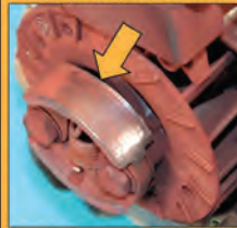
High Engine Load Worn Clutch Shoes
