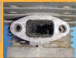
Partially Plugged Exhaust Port
