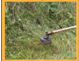
Heavy Engine Load No String Shield
