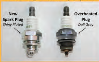
Overheated Spark Plug
