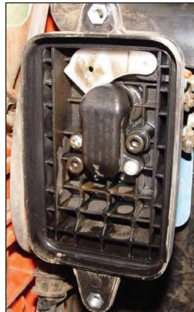
Check filter housing for dirt & debris
