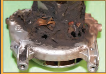
Blocked Engine Cooling Intake
