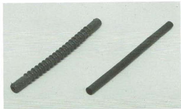
Left: Original impulse hose Right: New impulse hose
