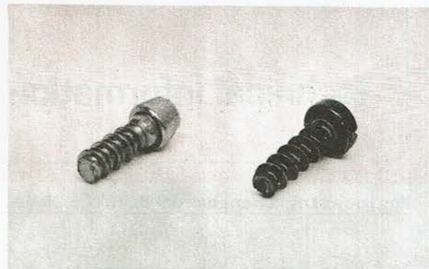
Mounting screws for annular buffer Left: Original version Right: New version
