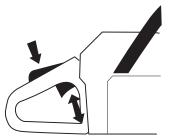
Start the chain saw and apply full throttle. Release the throttle control and check that the chain stops and remains stationary. If the chain rotates when the throttle control is in the idle position you should check the carburettor idle adjustment.
