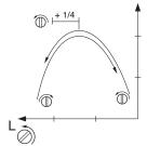
CAUTION! If the chain rotates while idling the T-screw must be turned anti-clockwise until the chain stops.
