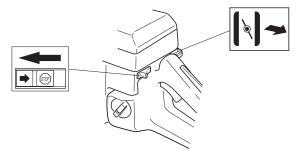
If the machine is fitted with a decompression valve (A): Press the valve to reduce the pressure in the cylinder and make starting easier. You should always use the decompression valve when starting the machine. Once the machine has started the valve will automatically return to its original setting.
