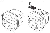
CAUTION! The muffler gets very hot during and after use. This also applies during idling. Be aware of the fire hazard, especially when working near flammable substances and/or vapours.
