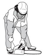
Push in the choke control as soon as the engine fires and keep pulling until the engine starts. When the engine
