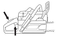
Note! Reactivate the chain brake by pushing the front hand guard back towards the front handle. The chain saw is now ready for use.
