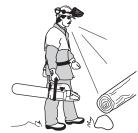
5 Take great care when cutting a tree that is in tension. A tree that is in tension may spring back to its normal position before or after being cut. If you position yourself incorrectly or make the cut in the wrong place the tree may hit you or the machine and cause you to
