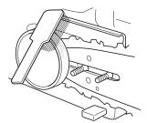
Regularly check that the brake band is at least 0.6 mm thick at its thinnest point.
