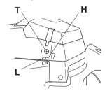
The L and H-jets are used to adjust the supply of fuel
