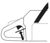
Press the throttle lockout and make sure it returns to its original position when you release it.
