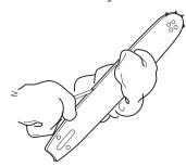
Check that the bar tip sprocket turns freely and that the lubricating hole in the tip sprocket is not blocked. Clean and lubricate if necessary.
