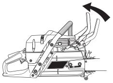
Remove the bar nuts and remove the clutch cover (chain brake). Take off the transportation ring (A).
