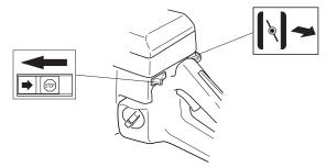
If the machine is fitted with a decompression valve (A): Press the valve to reduce the pressure in the cylinder and make starting easier. You should always use the decompression valve when starting the machine. Once
