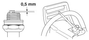
Note! Always use the recommended spark plug type! Use of the wrong spark plug can damage the piston/cylinder.
