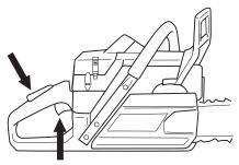
Note! Pull the front hand guard towards the front handle. The chain brake is now disengaged. Your saw is ready for use.
