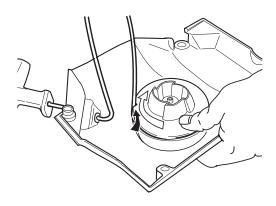
Undo the screw in the centre of the pulley and remove the pulley. Insert and fasten a new starter cord to the pulley. Wind approx. 3 turns of the starter cord onto the pulley. Connect the pulley to the recoil spring so that the end of the spring engages in the pulley. Fit the screw in the centre of the pulley. Insert the starter cord through the hole in the starter housing and the starter handle. Make a secure knot in the end of the starter cord.
