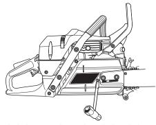
The chain is correctly tensioned when it does not sag from the underside of the bar, but can still be turned easily by hand. Hold up the bar tip and tighten the bar nuts with the combination spanner.
