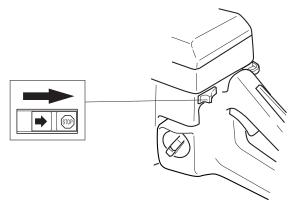
The engine is stopped by switching the ignition off using the stop switch.
