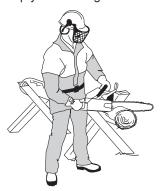
4 Never use the chain saw above shoulder height and avoid cutting with the tip of the bar. Never use the chain saw one-handed!
