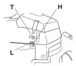
The T-screw regulates the throttle setting at idle speed. If the T-screw is turned clockwise this gives a higher idle speed; turning it anti-clockwise gives a lower idle speed.
