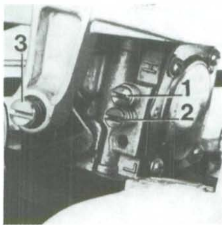
Fig. ST11—View of carburetor adjustment points typical of all models. High speed mixture needle (1) and low speed mixture needle (2) may be positioned differently on some models. Refer to text for adjustment procedure.
