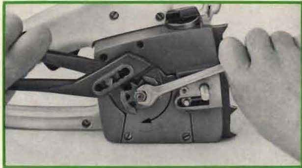
Top: Taking off the chain sprocket Bottom: Chain sprocket
