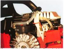
**Electronic Ignition System** for reliable starting. Completely enclosed. No problem with dirt or moisture.
