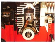
SOLO High-Performance Power Plant Specially coated cylinder walls, two piston rings, finely balanced crankshaft.
