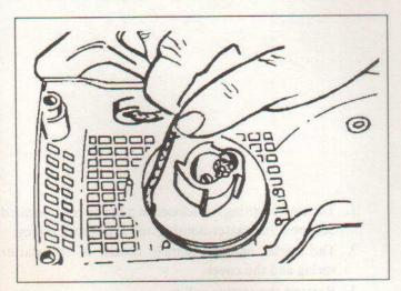
**NOTE:** If the starter rope requires replacement, yet is not broken, it is necessary to release the spring tension from the starter spring.
