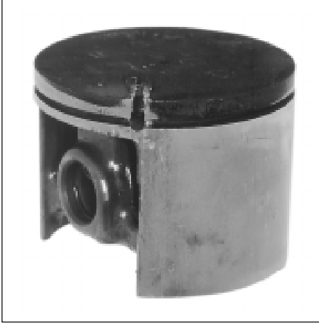
The guide pin for the piston ring has been pressed up through the piston head.
