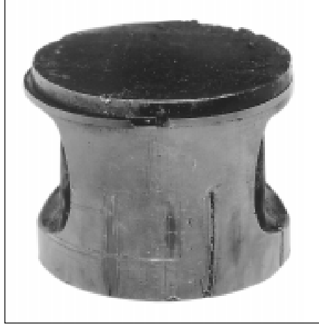
Deep and irregular grooves caused by a loose circlip. Here on the piston's inlet side.
