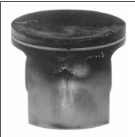
Inlet side. The piston ring has stuck in its groove. Black discolouring under the piston ring resulting from so-called "blow through".
