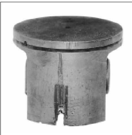
Severe damages to the lower part of the piston on the inlet side.
