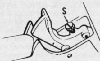
Fig. MC5-6—Adjust fast idle on models CP125, SP125 and SP125C by turning adjusting screw (S) on bottom of trigger.
