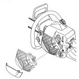
These reduce the flow of cooling air and prevent large amounts of snow from being sucked into the carburettor space.
