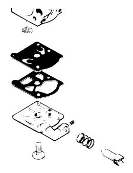
Assemble the fuel pump section. Press the fuel inlet screen into its seat evenly. Install the fuel pump diaphragm against the carburetor body first, followed by the gasket and cover.
