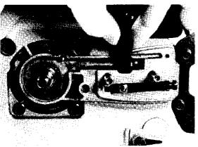
Using a screwdriver, carefully remove the oil suction tube and filter. Clean the oil pick-up filter.
