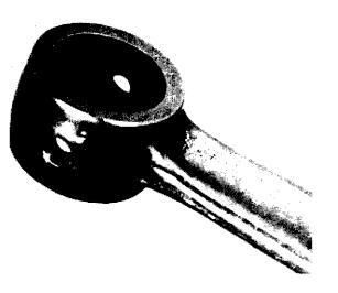
Check the small-end of the connecting rod. If seizure marks or discolored spots are evident in the bearing seat, the crankshaft must be replaced.
