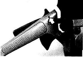
On the 50 and 50 Special models, the throttle lockout lever has a small tab midway on the left side. Insert a small screwdriver between the lever and lever opening on the left side so that the tab will clear the handle then withdraw the lever out through the top.
