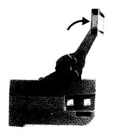
Clean chain brake and clutch cover assembly. Engage the chain brake by moving the hand guard forward.
