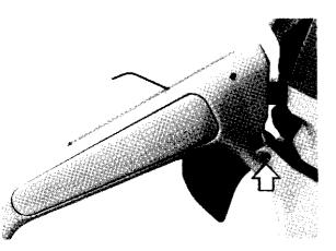
Drive out the pin for the throttle trigger. Raise the throttle trigger up into the handle and unhook the spring.
