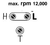
With the low speed mixture adjusted, the high speed mixture (screw H) is ready for adjustment. Run the engine at wide open throttle while observing the tachometer. Adjust the H screw so that the maximum no-load speed does not exceed 12500 rpm. After setting the high speed mixture, allow the engine to return to idle speed, then check for hesitation on acceleration. Repeat the complete final adjustment procedure of both the L and H mixture screws if necessary.
