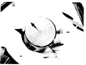
Position the piston over the connecting rod with arrow on the piston crown pointing towards the exhaust side. Align the piston pin boss holes with the connecting rod pin hole and install the pin. Carefully install the wrist pin clips ensuring that the clips are fully seated in the retaining grooves. Lubricate the piston and piston ring with oil.
