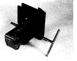
Mount the tool on the left crankcase half and press out the crankshaft.
