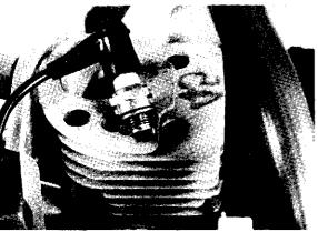
If no spark is evident, retest with a new spark plug or test plug P/N 5027113-01.
