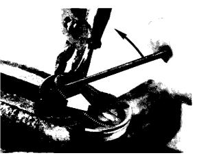
Secure the clutch hub in a vise. With the assistance of a screwdriver and a pair of pliers, lock the remaining clutch shoe so that the spring groove is exposed, then install the spring.
