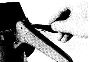
Insert the lockout lever making sure the end of the spring fits within the lever.
