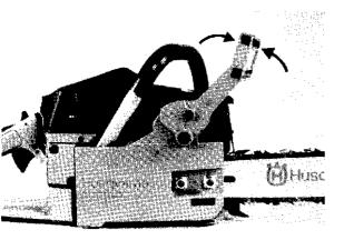
Mount the bar, chain and chain brake to the saw. Before running the saw, check the brake function by moving the hand guard forward until the brake engages. With the brake engaged, it should not be possible to rotate the saw chain around the guide bar. Pull the hand guard back towards the front handle to disengage the brake.
