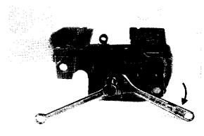
Install all the crankcase screws except the top front screw which also retains the bar spike and muffler support. Starting with the screws around the crankshaft, tighten all six screws to 7-9 Nm (5.1-6.6 ft.lbs.) torque.
