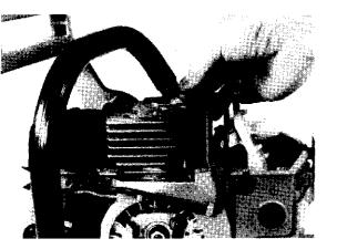
If the ignition module is new, it will be necessary to install a new spark plug connector spring on the high tension lead. Before installing the connector spring, first correctly route the high tension lead from the module to the spark plug. If necessary, cut the high tension lead to the correct length.
