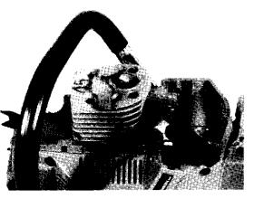
Remove the carburetor and intake manifold as described in section 10. Fuel System. Remove the spark plug and the exhaust system.
