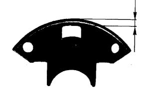
Inspect the clutch hub spokes for wear, Excessive wear causes a jarring sound and poor clutch operation.
