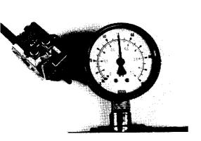
After assembly, pressure test the carburetor for air leaks. Pressure test at 50 kPa (7.2 psi). No air leaks are permitted.
