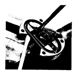
Check the clutch shoes for wear by measuring the material thickness at the shoes thinnest point. If the shoe is worn to less than 1 mm (0.040 in.) of material at the most worn part, the shoes must be exchanged.
