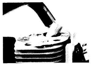
Gently rotate the flywheel counterclockwise by hand until the piston contacts the piston stop. Remove the flywheel retaining nut and washer. The flywheel nut has righthanded threads.
