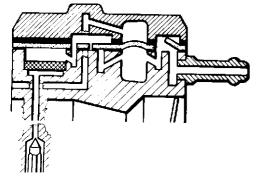
The pumping section consists of the fuel chamber and the diaphragm type fuel pump with the inlet and outlet check valves. The fuel pump draws the fuel from the tank to the fuel chamber, then pushes the fuel on to the metering section.
