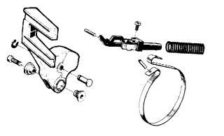
Check all chain brake parts for wear or damage and replace with new parts if necessary. Lubricate the linkage and pivots with thin oil.
