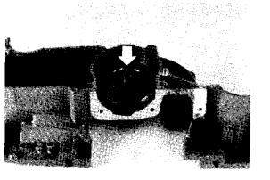
Heat the bearing seat area of the drive (left) side crankcase half and install the crankshaft bearing ensuring it is fully seated.
