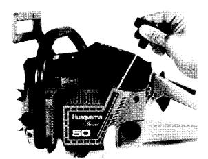
To install the starter assembly on crankcase, first pull the starter grip out approximately 15 cm (6 in.) then position the housing against the crankcase.
