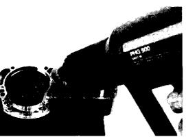
Remove the crankshaft bearings from the crankcase halves by heating up the crankcase around the crankshaft bearing then pressing the bearing out of the case.
