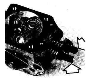
If the carburetor is very dirty it will be necessary to clean the fuel passages located underneath the fuel circuit plate (Walbro WA) or the welch plug(s) (Walbro WT).
