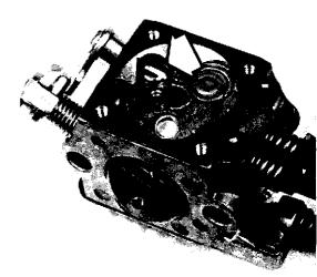
Check the needle valve. Replace a damaged or worn needle valve.
