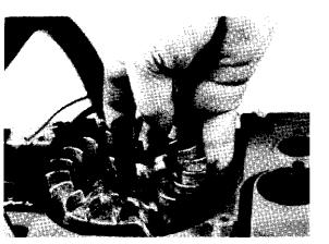
Hold onto the flywheel and lift the saw slightly above the work surface. Strike the tool squarely on its end with a hammer to free the flywheel from the crankshaft. Remove the tool and flywheel.
