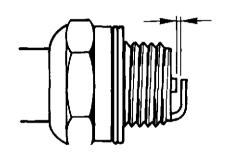
If the electrodes are worn, install a new, properly gapped spark plug.
