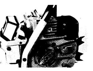
Rotate the clutch clockwise by hand until the piston contacts the piston stop. The clutch hub has left-hand threads. Loosen the clutch hub in a clockwise direction and remove the clutch.
