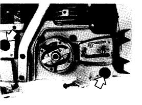
For access to the left side rubber elements, remove the starter housing.
