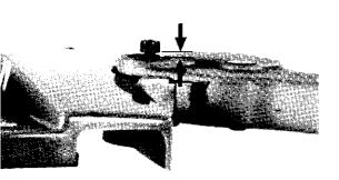
Remove hand guard retaining screw. Rethread screw into pivot sleeve two turns. Press on screw head to drive out pivot sleeve half on the opposite side.
