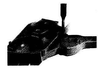
Remove the five screws and lift off the cover plate.
