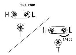
Turn the L screw back in to the mid-point between the lean and rich drop off settings, then open 1/4 turn. Adjust the idle speed to 2500-2800 rpm with the T screw again if necessary then recheck the L screw adjustment as previously described.
