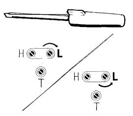
Begin with the low speed mixture screw. Using carburetor screwdriver P/N 5016002-02, turn the L screw in until the engine rpm's just start to decrease and note the screwdriver position. This is referred to as the lean drop setting. Now turn the L screw out until the engine rpm's just start to decrease again and note the screwdriver position. This is referred to as the rich drop setting.
