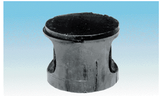
Deep, irregular grooves caused by a loose circlips is here shown here on the piston's inlet side
