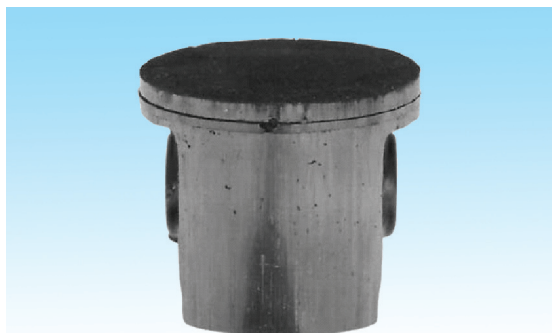
Particles of dust and dirt from carbon-like deposits on the top of the piston and in the piston ring groove
