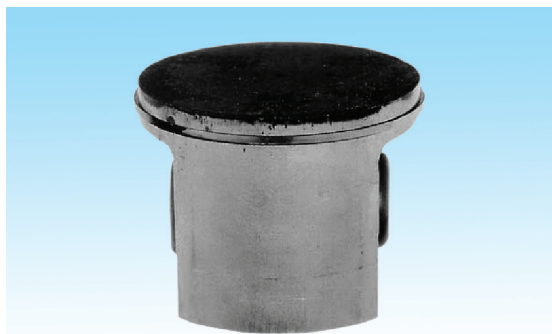
Small score marks and a matt, grey surface on the piston's inlet side caused by fine dust particles
