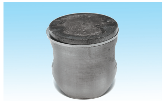
Piston from the exhaust side with normal wear and normal discolouring
