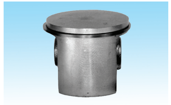
New piston from the exhaust side
