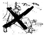
WARNING! Running an engine in a confined or badly ventilated area can result in death due to asphyxiation or carbon monoxide poisoning.
