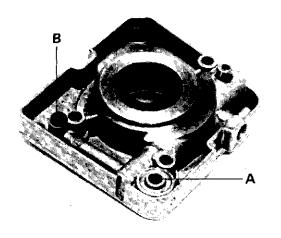
Check if there is dirt in the suction channel (A) by rotating the pump shaft in both directions. When the pump works properly and is filled with oil, the oil goes alternately through the suction channel and the compression channel (B).
