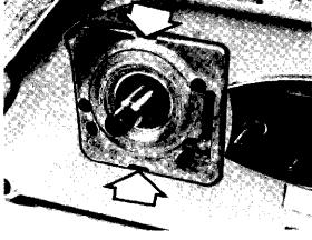
Remove the pump from the crankcase by levering around the edges of the housing with screwdrivers.
