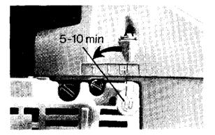
Screw in the H-needle slowly until there is no more fourstroking (position A). Then screw the needle out equivalent to 10 min on a clock-face.
