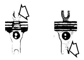
Check that the needle valve lever is not worn, neither at the connection to the needle valve nor the metering diaphragm.
