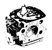
Loosen the screw that retains the bearing shaft of the lever and remove lever, shaft, spring and needle valve.
