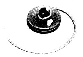
Pull the cord through the cord sleeve of the starter housing and through the starting handle. Make a knot in the cord and pull the knot completely into the handle. Put the cord into the groove of the pulley rim and tighten the spring enough to get 1/4 spare round. Fit the starter and check that no electrical cables are squeezed.
