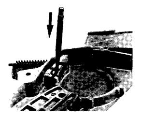
When dismantling the brake band use a drift Ø 4 mm to push out the roll pin.
