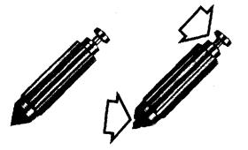
Check that the needle valve is not worn, neither on its seat, nor in the groove for the lever.
