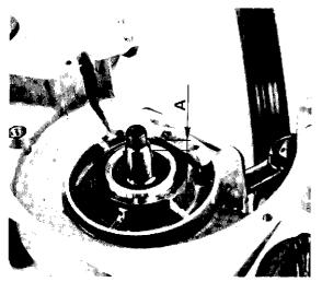
The distance between the sealing ring and the upper part of the seat (A) should be 3.5 mm. If less the flywheel will damage the sealing ring.
