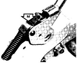
Loosen the nut (M) and lift off the hand guard.
