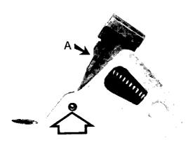
The catch may be changed after pushing out the roll pin with a drift  $\emptyset$  4 mm. Check the wear on the locking part of the catch (see A).
