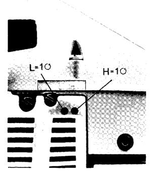
After having made the abovementioned checks you make a basic adjustment of the carburettor needles, i.e. H = 1 turn open and L = 1 turn open.
