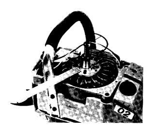
Fit holding bar No. 50 25 149-01 on the flywheel and loosen the nut with a box spanner (14 mm). Fit puller No. 50 25 026-01 on the holding bar and remove the flywheel.
