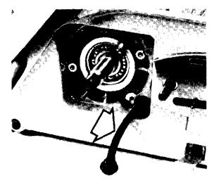
Lift the suction hose and oil filter out of the oil tank. Clean the parts and change any that may be damaged.
