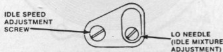
Fig. HL41-1—View showing location of idle mixture screw (I) and idle speed screw (S).
