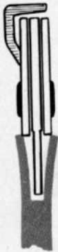
Fig. HC2— Chain will not run true in spread guide bar rails.
