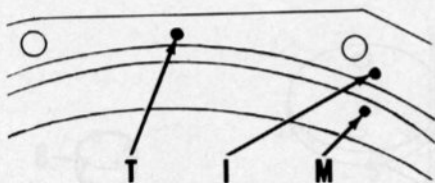
Fig. L4-5—Drawing of flywheel timing marks used on some models.
