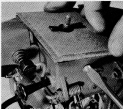
Fig. HL4—Before tightening screws retaining air filter bracket in throttle handle, place air filter element on bracket stud and align filter with edges of air box.
