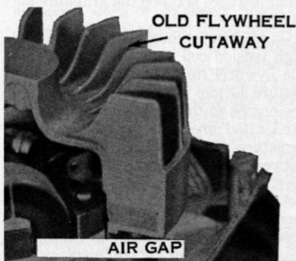
Fig. S38 —Where armature core and ignition coil are located inside of flywheel, an old discarded flywheel can be cut away as shown to provide air gap adjustment fixture.
