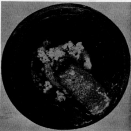
Fig. S5—Core bridging from center electrode to shell. Fused deposits sometimes have the appearance of tiny beads or glasslike bubbles. Caused by excessive combustion chamber deposits which in turn could be the result of: excessive carbon from prolonged usage; use of improper oil or incorrect fuel-oil ratio.
