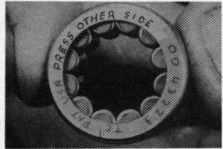
Fig. HL9—Roller type main bearing used at flywheel end of crankshaft is marked on one side, "PRESS OTHER SIDE". Be sure to observe this precaution when installing bearing in crankcase.
