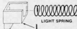
Fig. HL29-2—Note position of lug (L) when identifying high and low speed sliders. Be sure correct spring is installed in slider.
