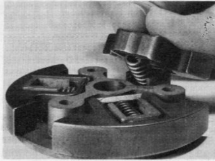
Fig. HL44-7—Installing shoes and springs on clutch spider plate.
