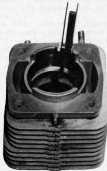
Fig. S48—Clearance between ends of ring (ring end gap) should be measured with feeler gage as shown. Make sure ring is straight in cylinder.
