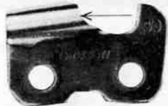
7. Backslope on side plate.
