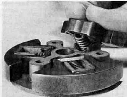
Fig. HL118 —To install clutch shoes, hook shoe and spring on clutch plate as shown, then push shoe down into place. Early type clutch is shown.
