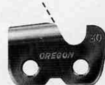
Backslope in side plate—caused by holding file too high. Chain won't feed properly; cutters wear fast at heel.
