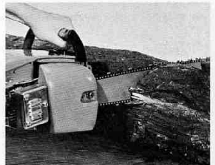
6. Use extra oil first half-hour of cutting with new chain.
