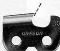
Hook in side plate—caused by pressing file down too hard, or holding file too low.
