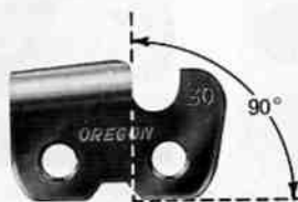
90° Side Plate Angle—Chipper, Micro-Bit, Micro-Guard.
