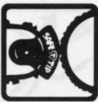
3. THE SAFE•T•TIP® DEVICE ON YOUR BAR NOSE PREVENTS KICKBACK.
