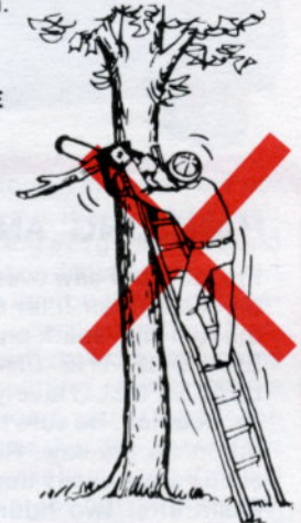
CUTTING ALOFT OR FROM LADDERS IS EXTREMELY DANGEROUS.
