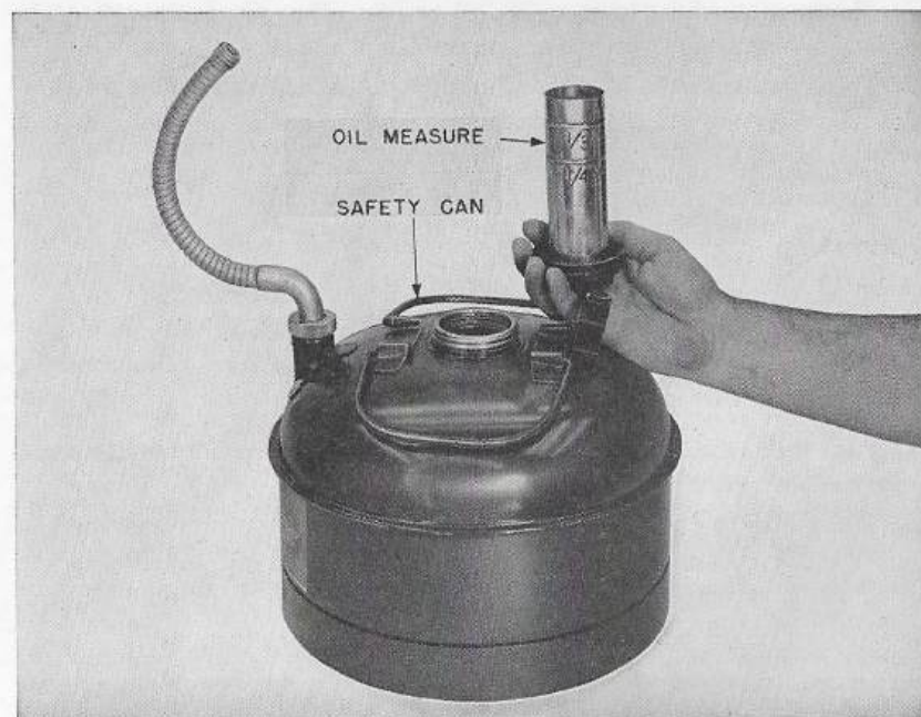
Figure 3—Mixing Gasoline and Oil in Homelite Safety Can
