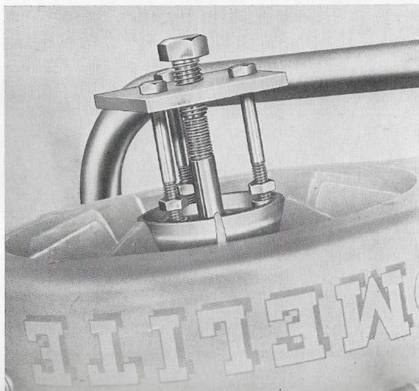
Figure 18—Pulling Magneto Rotor
