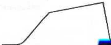
If tooth is shaped to pull away—Negative Hook. For hard or frozen wood.
