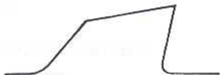
If tooth is shaped to dig in—Positive Hook.
