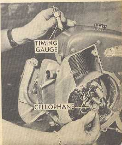
A cellophane strip and this gauge make the ignition timing simple.
