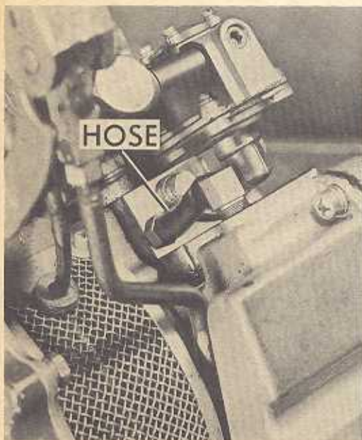
Make sure this hose connection is leak-proof
