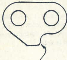
TANGS HAVE ROUNDED, OR DULLED FRONT CORNERS
