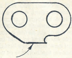
TANG BOTTOMS ARE SHARP, FLAT, WORN PARALLEL TO BAR
